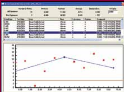
On-the-fly trending of any test point. Historical values are shown in blue with connecting lines. Values for similar equipment are shown in red. A table above the trend chart lists all of the data values, along with the test date and equipment location.
